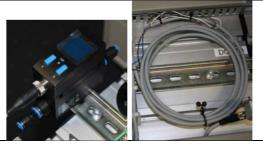
Measure the air flow for the whole system. Connect only the 24V/0V to the I/O-Terminal in the station Don't cut the cable short (keep it as ring)
